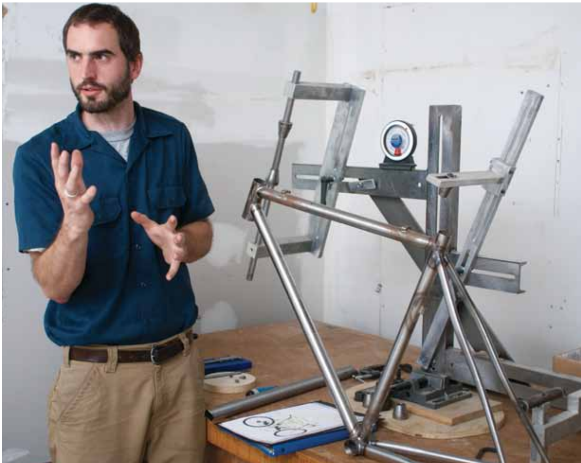
(Above) Eric Kritivzky, owner of Penguin Cycles in Brownsville, Vt., by the frame jig he uses in his workshop.
